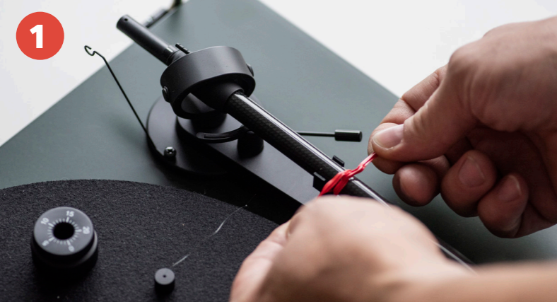
1 Remove the counterweight and anti-skating weight from the tonearm. Secure the tonearm using the supplied red wire.
