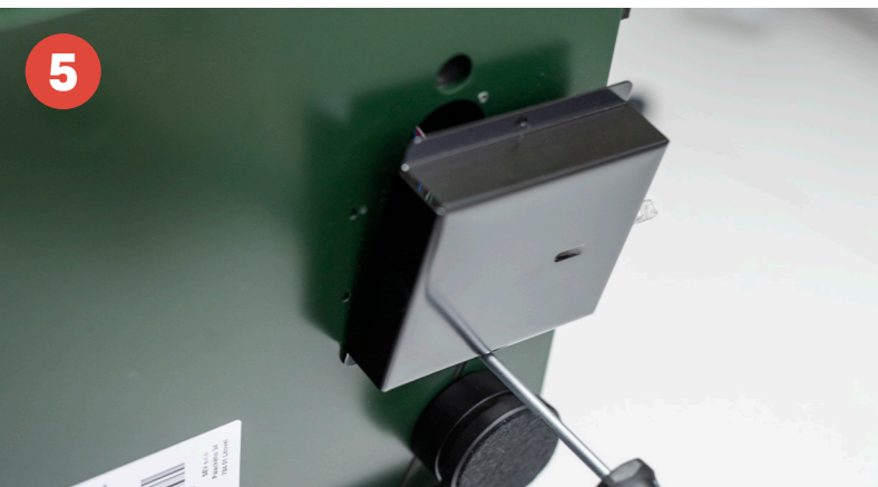
5 Loosen the lower screw just a little to be able to rotate the RCA box.
