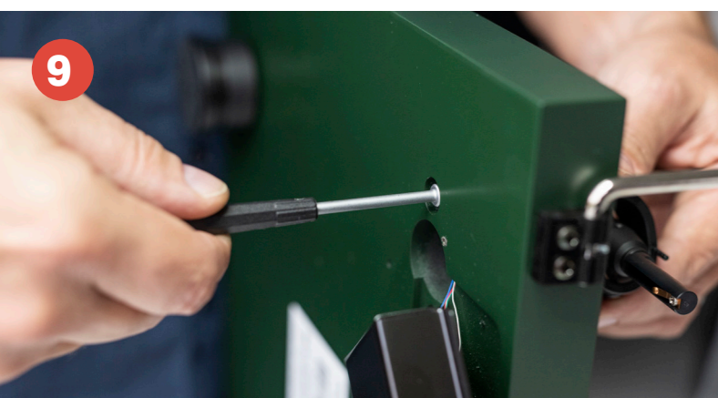
9 Loosen the upper nut by 3mm.
